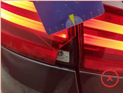
E.g. Broken lamp unit
