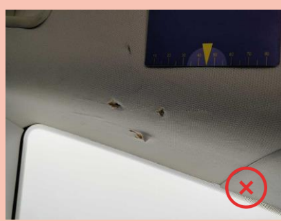
E.g. Holes in the ceiling fabric
