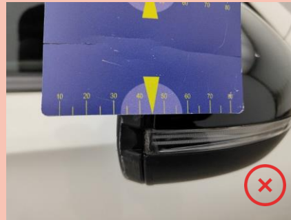
E.g. Broken side indicator light
